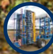
BÂTI PORTEUR SÉCURISÉ, REPLIAGE HYDRAULIQUE
